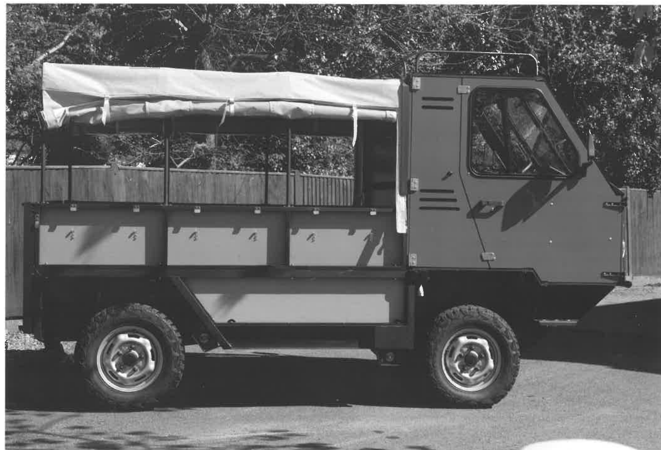
The prototype of the OX, a lightweight flatpack truck engineered to be a cheap method of long distance transport and travel even on rigorous African roads.
