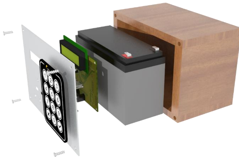
FIGURE 58 - EXPLODED VIEW OF FULL IZUBA.BOX DESIGN
