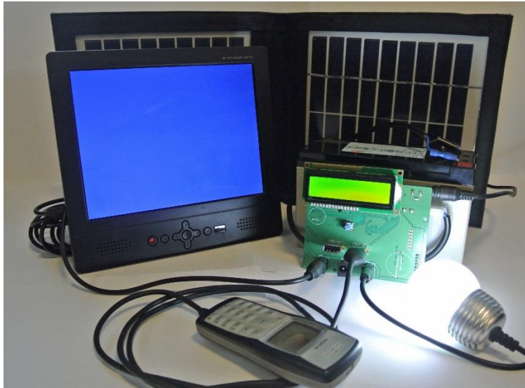
FIGURE 51 – PROTOTYPE SYSTEM POWERING TV, LED LIGHT AND CHARGING A MOBILE PHONE
